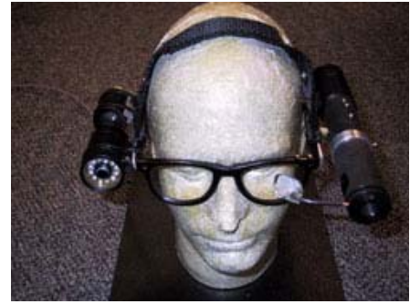
The head-mounted components of the Wearable Low Vision Aid. Shown are the camera with a ring of infra-red LEDs (left) and the head mounted display (right).
