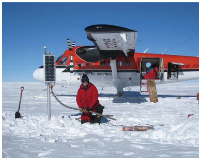
Polar engineer Guy Tytgat installing a seismographic station in Antarctica's Gamburtsev Province. Credit: IRIS.
