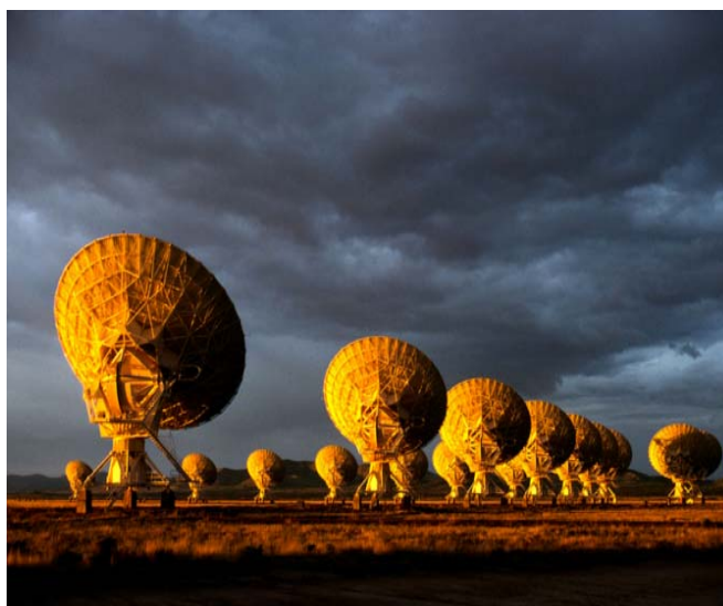
In 2010 the Very Large Array (VLA) telescope, located about 80 km west of Socorro, NM, transformed into the Expanded Very Large Array (EVLA). Like the VLA the EVLA is composed of 27 individual antennas arranged in a "Y" pattern. In their closest configuration (about 1 km wide), the EVLA is able to image large portions of the sky. In its largest configuration (about 36 km wide) the EVLA is able to home in on the fine details of astronomical objects. Credit: Andrew Clegg, National Science Foundation.
