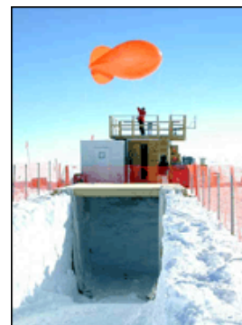
A researcher attaches an instrument to a tethered balloon to measure the characteristics of water vapor in the lower two kilometers of the atmosphere at Amundsen-Scott South Pole Station, Antarctica. (NSF/USAP photo by Jeff Ingles, Raytheon Polar Services Corp.)
