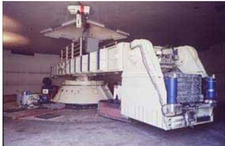
Nine-meter centrifuge at the Center for Geotechnical Modeling at UC Davis, a host facility in the Network for Earthquake Engineering Simulation, funded by the National Science Foundation.
