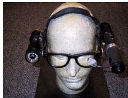
The head-mounted components of the Wearable Low Vision Aid. Shown are the camera with a ring of infra-red LEDs (left) and the head mounted display (right).
