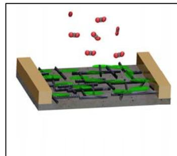
Conceptual illustration of the carbon nanotube network device coated with poly (ethylene imine) and starch polymer layer for detection of CO<sub>2</sub> gas
