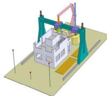
Diagram of the construction of a conventional building using Contour Crafting.
