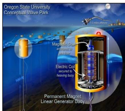
Ocean buoy generators promise to convert the movement of waves into energy.
