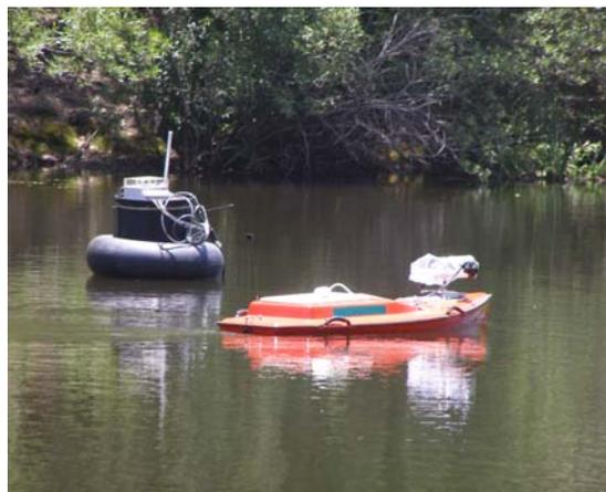
Robotic Aquatic Observing System. Credit: Center for Embedded Networked Sensing (CENS).
