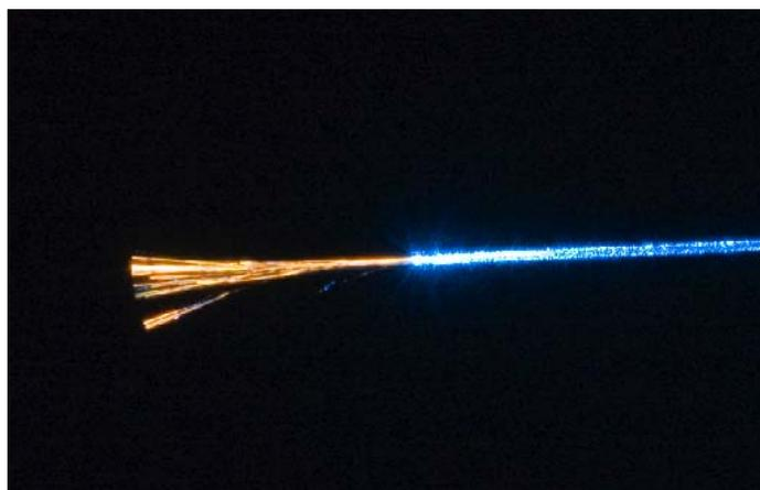
A wire-packed glass fiber. Each of the semiconductor wires is just two micrometers in diameter – 1/20<sup>th</sup> the width of a human hair. *Credit: Neil Baril, Penn State University.*
