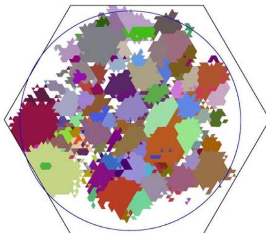
A two-dimensional slice of the microstructure inside of an aluminum wire, 1 mm in diameter (the blue circle). Each color corresponds to a different crystal orientation. *Credit: R.M. Suter, MRSEC, Carnegie Mellon University.*
