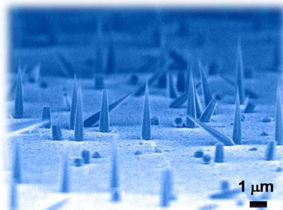
Nanolasers grown on a silicon substrate integrate easily into integrated circuits. Scale: 1 micron.
