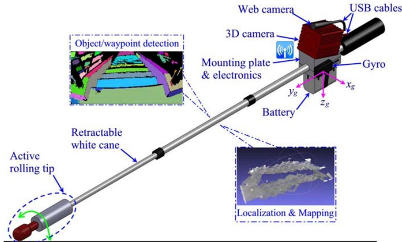
At the University of Arkansas at Little Rock, researchers prototyped a robotic walking stick for the blind. It has cameras to detect objects in the way such as chairs and stairs, an audio system that communicates to the user, and a computer that remembers recent pathways and objects in them. Developed under the National Robotics Initiative, a multi-agency program partnership that includes NSF.
