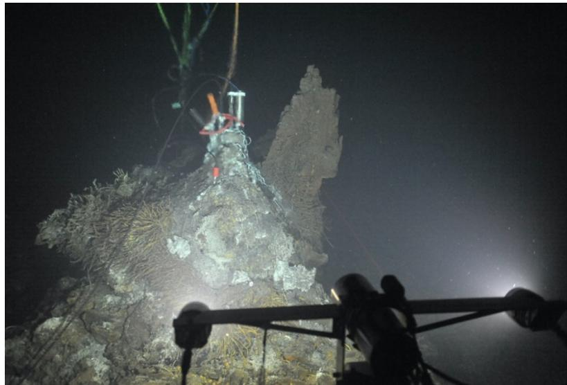
The Regional Cabled Array cabled digital still camera, redeployed in 2015 by the Canadian ROV ROPOS, lights up the active hydrothermal vent called El Gordo in the international District Hydrothermal Field, located at the summit of Axial Seamount nearly a mile beneath the ocean surface. *Credit: UW/NSF-OOI/CSSF.*
