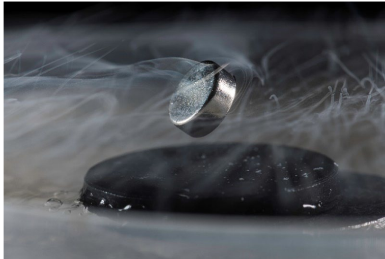
The goal of new research is to develop room temperature superconducting materials. Currently, extreme cold is required to achieve superconductivity, as demonstrated in this photo in which a magnet floats over a superconductor cooled in liquid nitrogen. Credit: University of Rochester / Adam Fenster.
