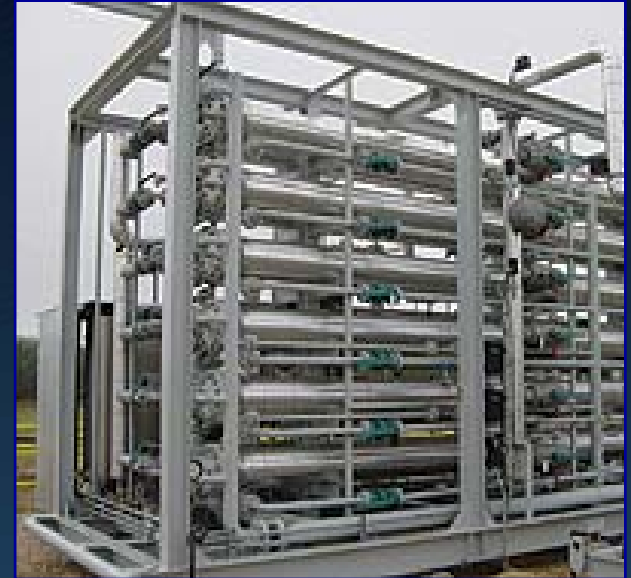
Polaris™ membranes remove CO 2 from Syngas. Credit: MTR
