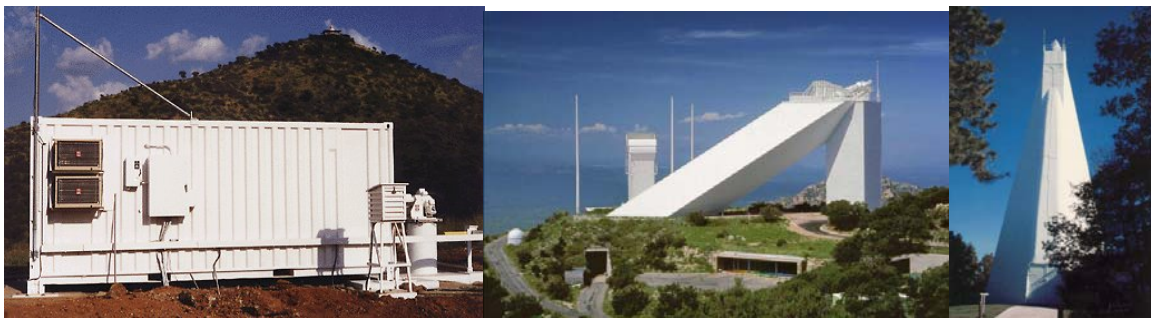
Figure 14. (a) On the left is the NSO’s Global Oscillations Network Group (GONG++) facility at Udaipur, India. This is one of six such installations around the globe used for near-continuous observations of the sun. GONG is a fundamental instrument for the study of solar oscillations and subsurface gas flows and was one of the pioneer instruments in the field of helioseismology. (b) In the center is the NSO site on Kitt Peak near Tucson, AZ. The large tower and angled structure is the McMath-Pierce Telescope. With a 1.6-m aperture, the McMath-Pierce Telescope is the world’s largest solar telescope. The vertical structure to the right is the former Kitt Peak Vacuum Telescope and is now the home of the SOLIS telescope. (c) On the right is the NSO site on Sacramento Peak near Sunspot, NM. The large tower houses the Dunn Solar Telescope (DST). The tower rises 41.5m above the ground and the optical system extends 67m below ground. The DST forms an image of the sun 51-cm across. The DST offers a routine adaptively-corrected feed and is the test bed for many of the instrument concepts that will be incorporated into the ATST. [Image credit: NSO/AURA/NSF]
