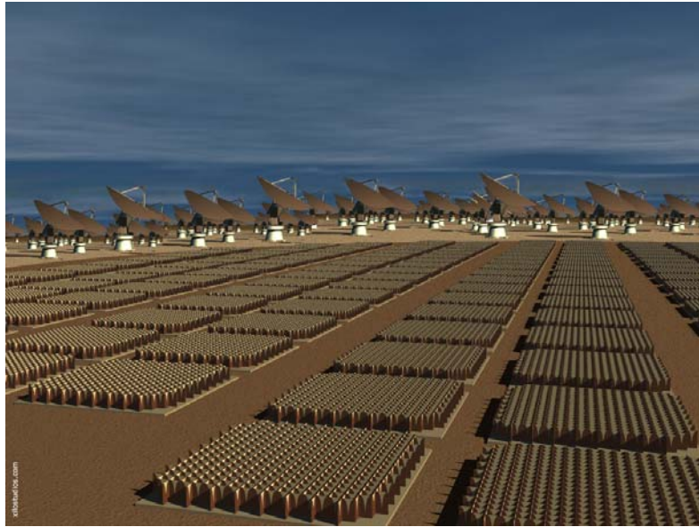
Figure 18. The Square Kilometer Array (SKA) is being planned by an international group of scientists and engineers as a next-generation facility for observations from 30 MHz to 30 GHz. This artist's conception shows aperture array (front) and small telescope (back) designs that are currently being considered to cover this broad frequency range. Sites in Australia and South Africa are under consideration. [Image credit: Xilostudies]
