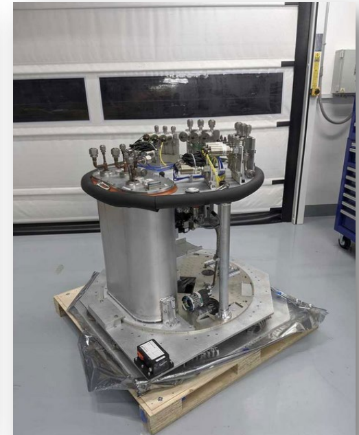
Refrigeration pathfinder unit built at SLAC and delivered to the summit (Feb 2020)
