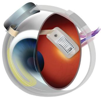
damage, researchers at the **Center for Biomimetic Microelectronic Systems (BMES)** developed an artificial retina. Spun off through Second Sight, a medical products company, the Argus® II retinal prosthesis became the first medical device to earn U.S. Food and Drug
