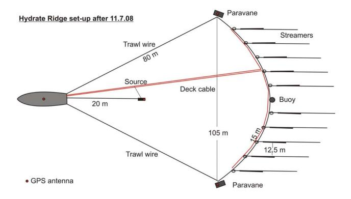
FIGURE 2.2. Towing configuration of the two GI guns and the P-Cable system (10 streamers shown) during the NEPO seismic study, 30 June to 19 July 2008.
