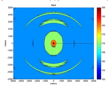
Figure 10.4. Closer view of broadband propagation field, run out to < 170 dB isopleth.
