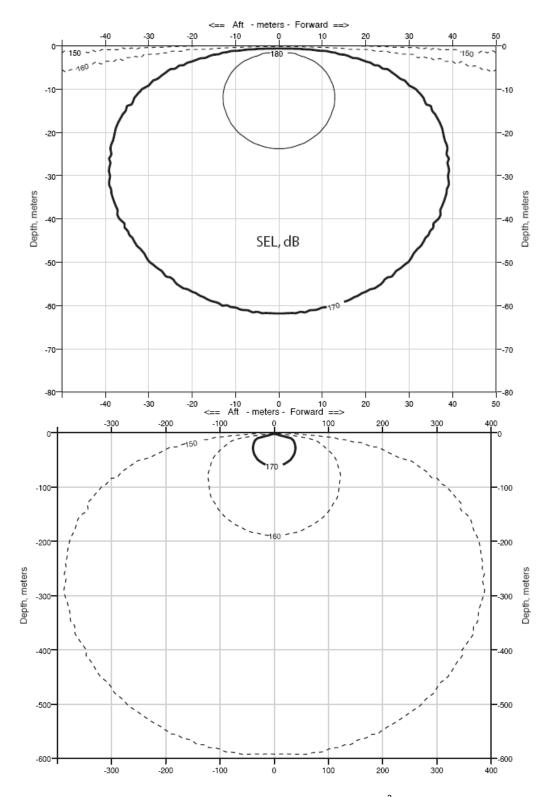
FIGURE 3. Modeled received sound levels (SELs) from a single 40-in<sup>3</sup> airgun operating in deep water, which is planned for use as a mitigation airgun. Received rms levels (SPLs) are expected to be ~10 dB higher.
