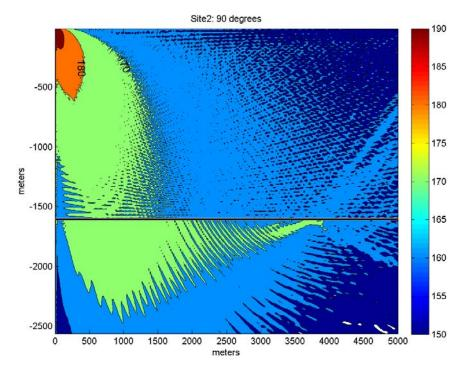
Figure 8.2. Transmission Loss along 90° radial (athwartship), contoured into 10 dB steps.
