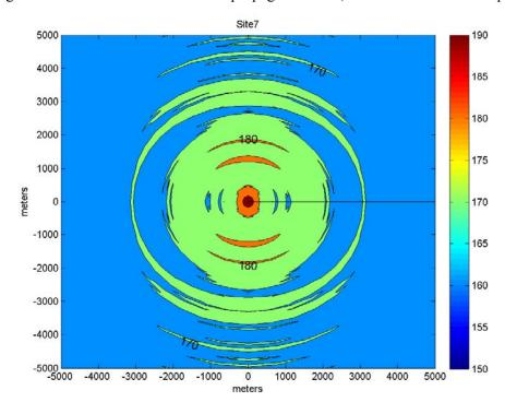
Figure 13.4. Closer view of broadband propagation field, run out to < 170 dB isopleth.
