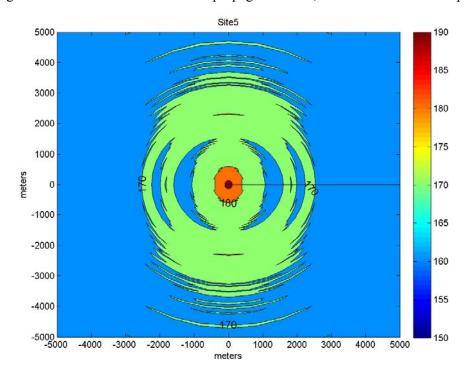
Figure 11.4. Closer view of broadband propagation field, run out to < 170 dB isopleth.
