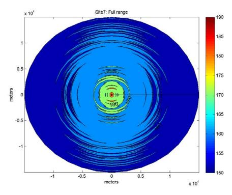
Figure 13.3. Plan view of broadband propagation field, run out to < 160 dB isopleth.
