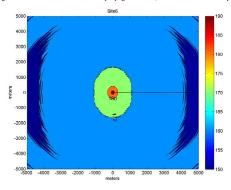
Figure 12.4. Closer view of broadband propagation field, run out to < 170 dB isopleth.
