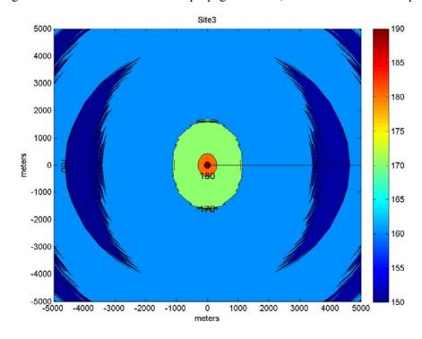
Figure 9.4. Closer view of broadband propagation field, run out to < 170 dB isopleth.
