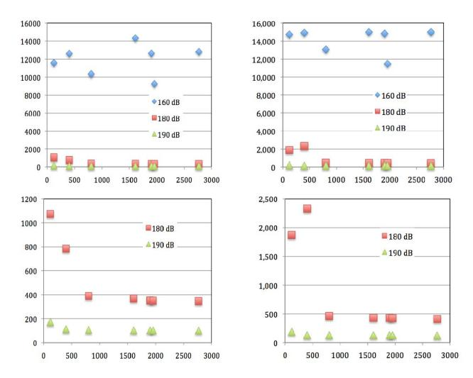
FIGURE 6. The mean (left column) and 95<sup>th</sup> percentile (right column) radial distances to the different isopleths are shown as a function of water depth. The top row shows the 160, 180 and 190 dB isopleths, while the bottom row shows only the 180 and 190 dB isopleths. Despite the differences in seafloor properties, water depth appears to be the driving factor in determining the range to different isopleths.
