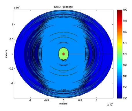
Figure 8.3. Plan view of broadband propagation field, run out to < 160 dB isopleth.
