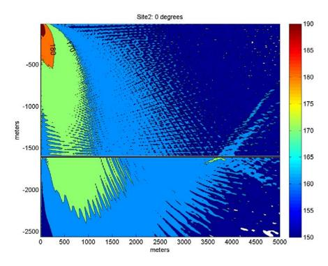
Figure 8.1. Transmission Loss along 0 degree radial (fore-aft), contoured into 10 dB steps.
