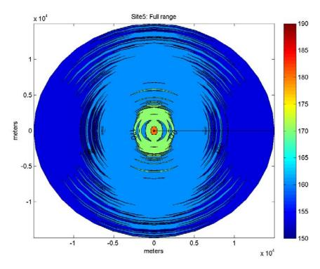
Figure 11.3. Plan view of broadband propagation field, run out to < 160 dB isopleth.
