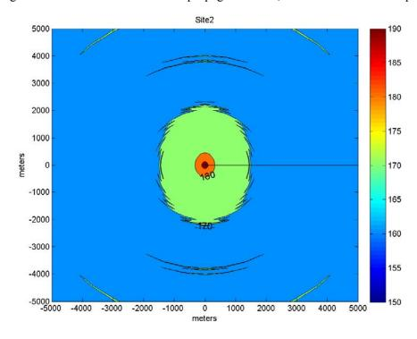
Figure 8.4. Closer view of broadband propagation field, run out to < 170 dB isopleth.
