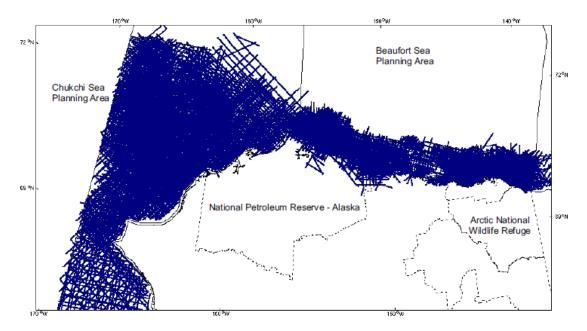
Figure 6. 2-D seismic survey lines shot in the Chukchi Sea and Beaufort Sea planning areas during 1980–1989. Source: MMS.
