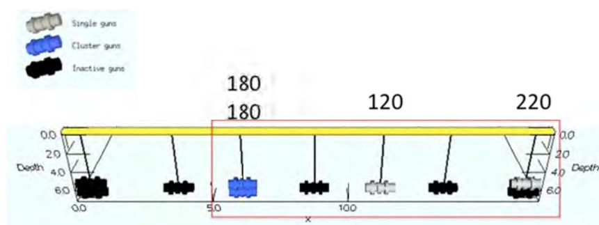
FIGURE A1. Four-airgun subset of one string that would be used as a 700-in 3 subarray for the proposed survey (individual volumes are indicated).
