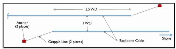
Figure 2-23. Proposed Cable Laying at Node Locations – Overlapping Segment End Method
