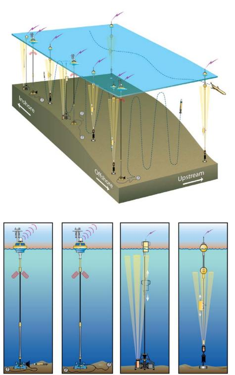
Figure 2-9b. Schematic Diagrams of the Proposed Pioneer Array (top) and Moorings (bottom) as Assessed in this SSEA
