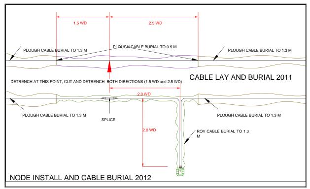
Figure 2-26. Proposed Cable Laying at Node Locations – Straight Continuous Piece Method
