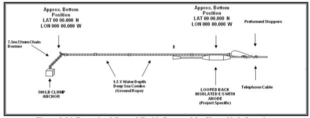
Figure 2-24. Example of Ground Tackle Proposed for Use at Node Locations
