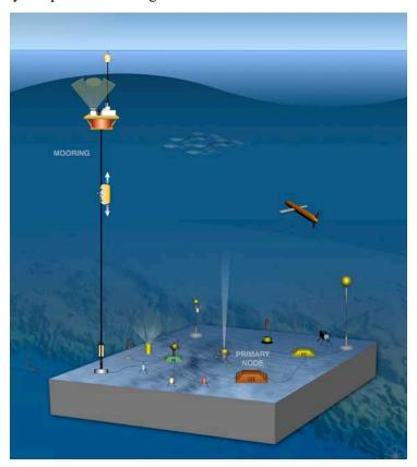
Figure 2-11. Conceptual Representation of a Hybrid Profiler Mooring
