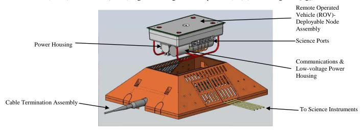
Figure 2-10. Trawl-resistant Frame (TRF) for Primary Nodes
