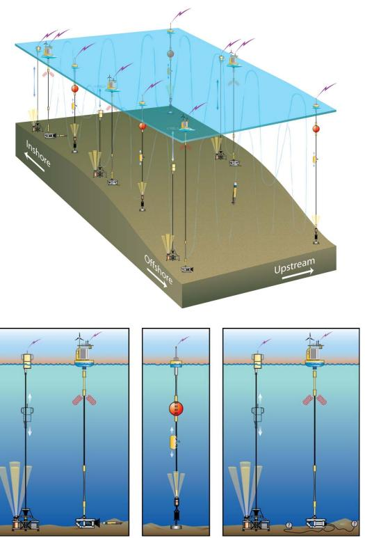
Figure 2-9a. Schematic Diagrams of the Pioneer Array (top) and Moorings (bottom) as Previously Assessed in the PEA and SER
