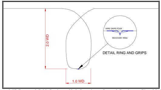
Figure 2-27. Proposed Cable Laying at Node Locations – Looped Continuous Piece Method
