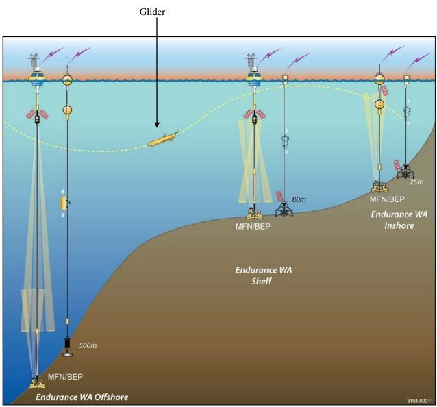
Figure 2-2. Conceptual Representation of the 25-m (Inshore), 80-m (Shelf), and 500-m (Offshore) Moorings of the Proposed Endurance Array (Grays Harbor Line)
