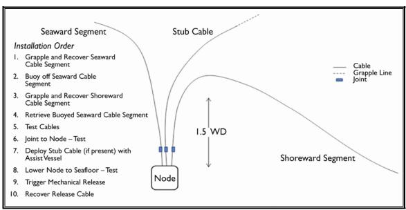
Figure 2-25. Proposed Node Installation – Overlapping Segment End Method
