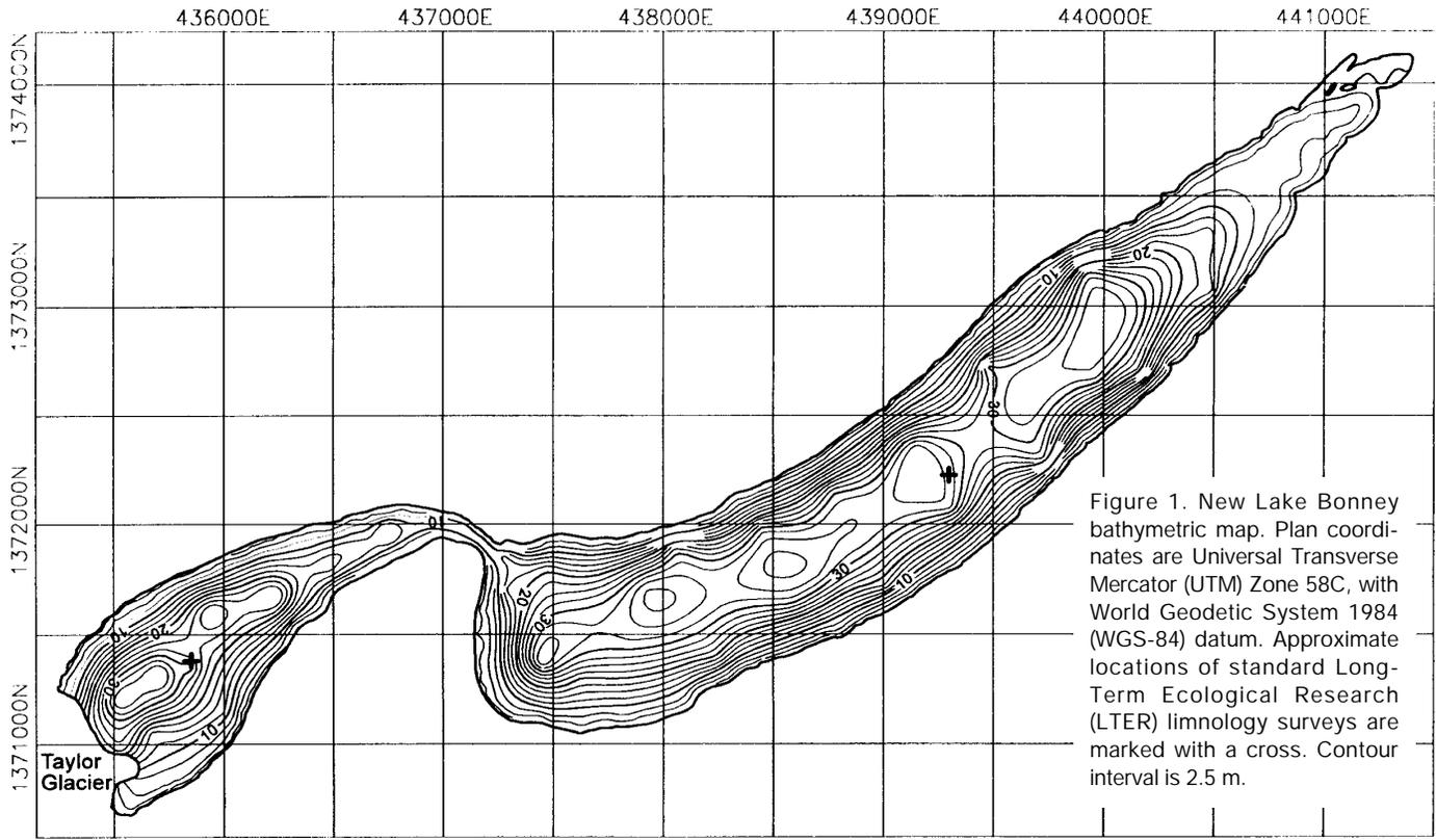
Figure 1. New Lake Bonney bathymetric map. Plan coordinates are Universal Transverse Mercator (UTM) Zone 58C, with World Geodetic System 1984 (WGS-84) datum. Approximate locations of standard Long-Term Ecological Research (LTER) limnology surveys are marked with a cross. Contour interval is 2.5 m.
