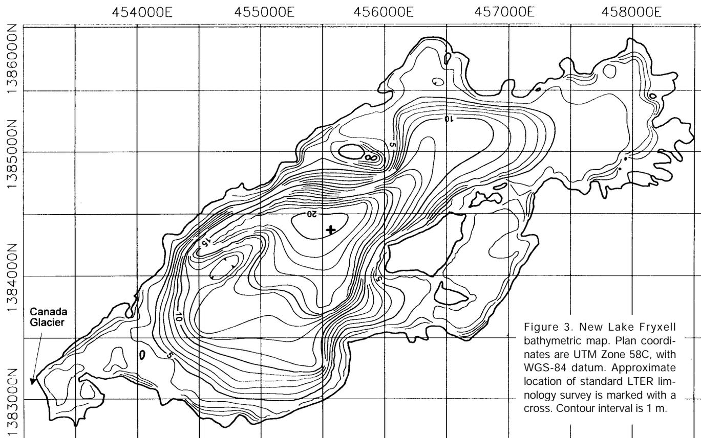
Figure 3. New Lake Fryxell bathymetric map. Plan coordinates are UTM Zone 58C, with WGS-84 datum. Approximate location of standard LTER limnology survey is marked with a cross. Contour interval is 1 m.
