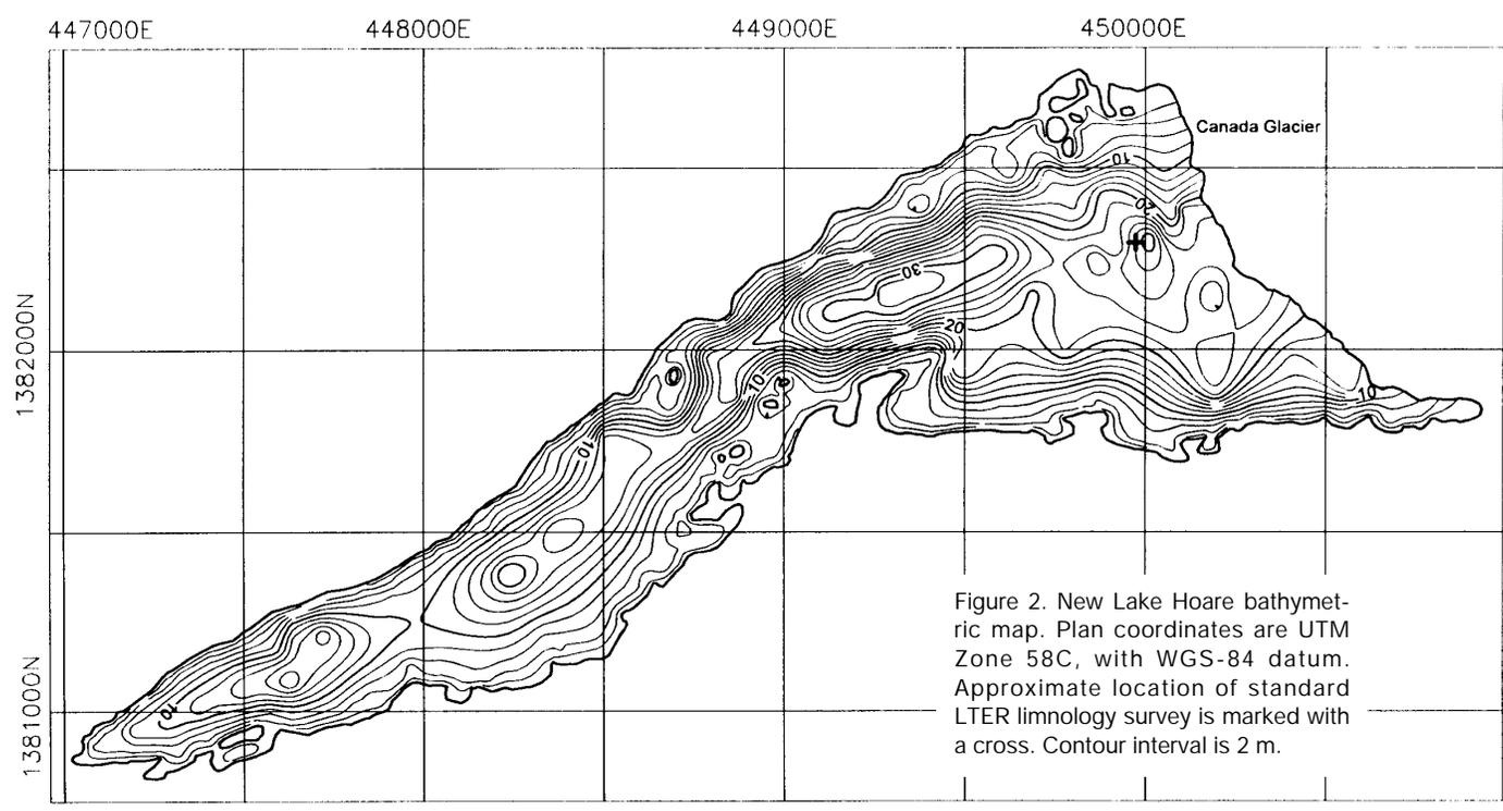
Figure 2. New Lake Hoare bathymetric map. Plan coordinates are UTM Zone 58C, with WGS-84 datum. Approximate location of standard LTER limnology survey is marked with a cross. Contour interval is 2 m.
