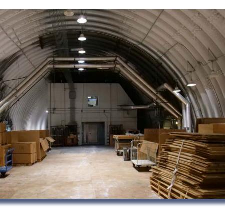
WAREHOUSING IN THE LOGISTICS ARCH. The logistics arch and heated warehouse building have a structural steel and plywood floor to allow the forklift use and pallet storage; the floor is beginning to dome. Source: NSF,
