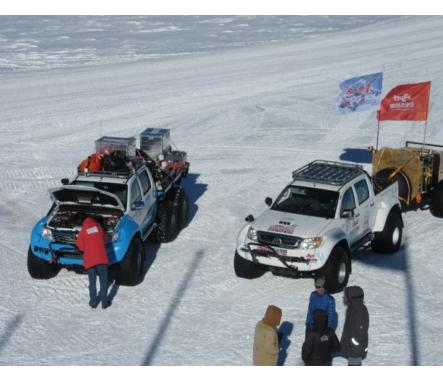
AGILE OVERLAND TRAVERSE. Small overland traverse vehicles have been used in Antarctica in the past and may be a cost and time saving alternative to field flights in crevasse-free areas. Source: NSF, Undated.
