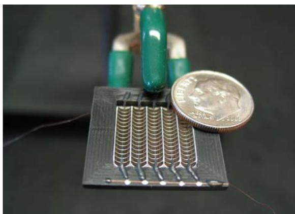
Researchers have developed a new micro-fan only slightly larger than a dime. The new fan can generate winds on the same scale as a laptop computer fan, but uses far less energy. Credit: Dan Schlitz and Vishal Singhal, Thorn Micro Technologies
