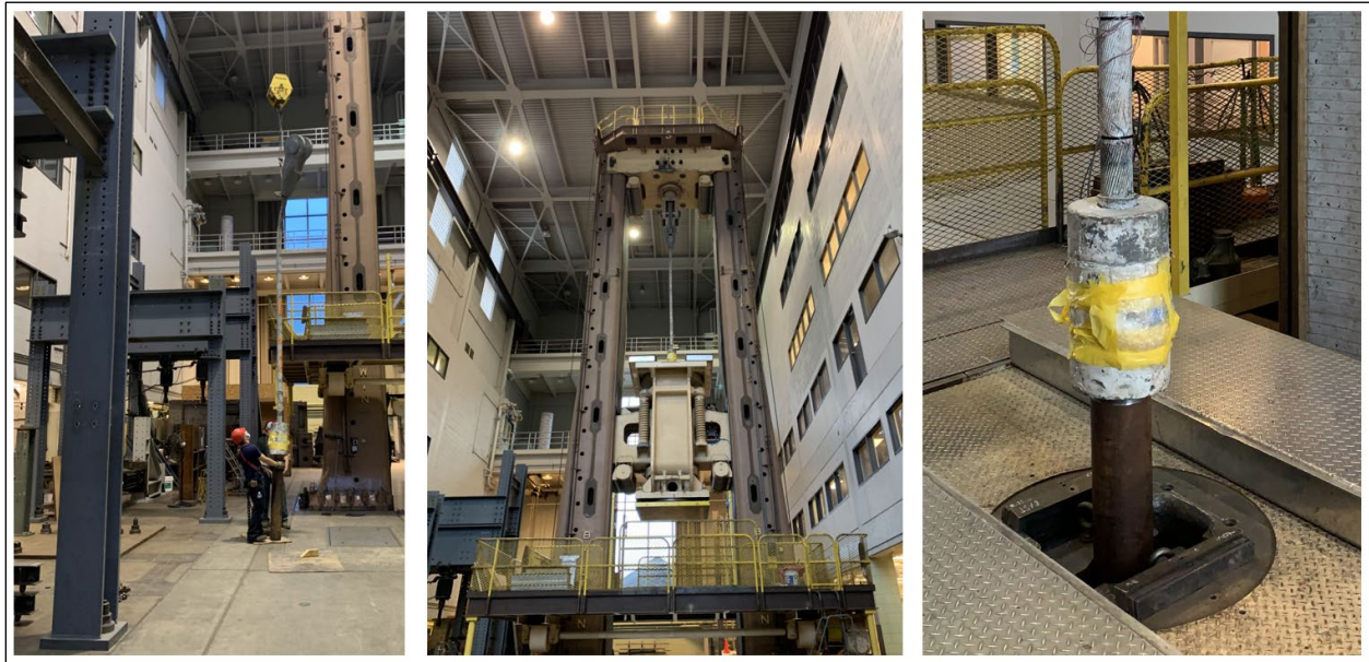
Figure 7: Cable test at Fritz Laboratory using a 5,000-kip universal testing machine.
