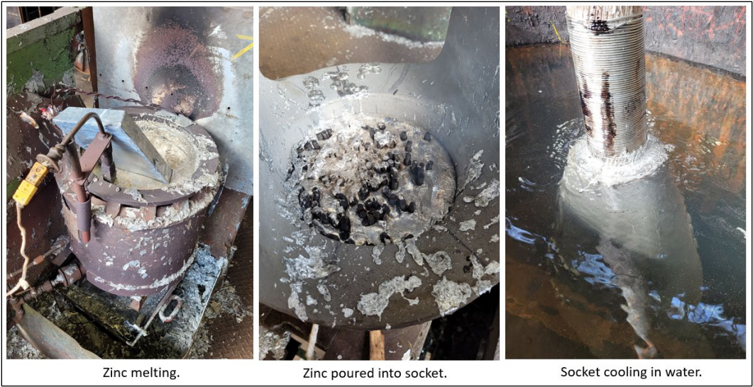
Figure 6: Zinc casting and socket cooling.
