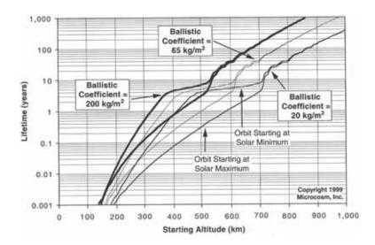
Figure 18: Figure 8.4 from Satellite Mission Analysis and Design [42] shows the reentry time from atmospheric drag for various ballistic coefficients.
