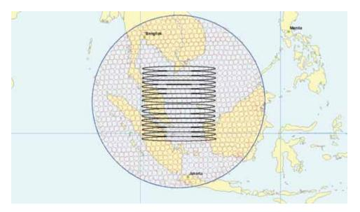
Figure 11: Beam footprints in Ku-band for internet service provided by LEO satellites (Starlink in orange, OneWeb in black ). Beam footprints in Ka-band will be 3 times smaller, or as small as 20 km. From [44].
