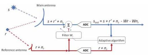
Figure 14: Same as Figure 13 except that the two signals pass through an ADC (analog-to-digital converter), pehaps to low bit depth b, before correlation.
