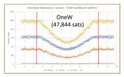
Figure 6: Example calculation taken from Patrick Seitzer talk to JASON. The figure shows the visible number of OneWeb satellites for a constellation size of 47,844, for summer observations at Cerro Tololo. Note that over 500 satellites in three planes would be visible even at midnight. Yellow indicates the total number of satellites over all planes; blue, orange, and gray specifies the orbital planes with inclinations 40, 55, and 87.9 degrees respectively. See also [37].
