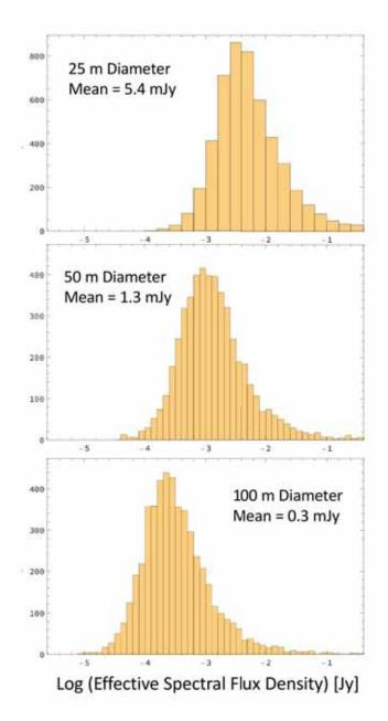
Figure 12: Estimated distributions of power spectral density from a telescope pointed at 45 degrees zenith angle. The telescope will see a different RFI contribution level approximately every minute, sampled from the indicated power spectral density distributions. Distributions are for telescopes of 25, 50, and 100 meters in diameter, and a total constellation size of 40,000.
