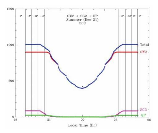
Figure 3: A simulation from J. McDowell showing the number of illuminated satellites from the OneWeb and Starlink Phase 2 constellations at the summer solstice. Even in the middle of the night over 400 satellites (all from the OneWeb constellation) are illuminated and visible from the Rubin Observatory.
