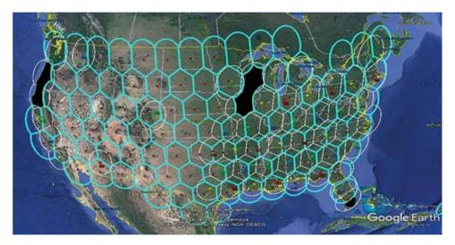
Figure 10: Beam footprints in Ka band for internet service provided by a GEO satellite (HughesNet Corp, in teal); each is about 300 km across. GEO satellite transmissions are generally moving from Ku band to Ka band. From [25]
