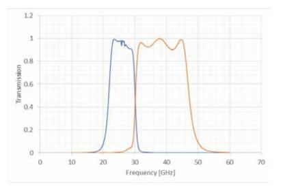
Figure 16: The low frequency filter bands of the Simons Observatory.
