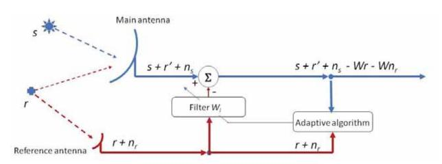
Figure 13: The astronomical signal s is corrupted by RFI from a satellite signal r. The reference antenna captures signal r from the satellite. An adaptive filter W then cancels the RFI by subtracting Wr = r from s, with accuracy limited by noise  $n_s$  and  $n_r$ .
