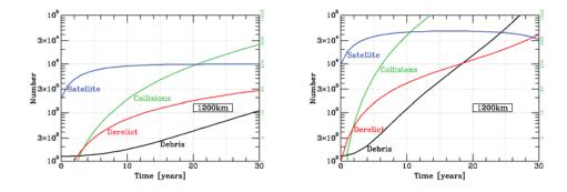
Figure 21: The solution of Equation 5-22 for  $\lambda = 2000/\text{yr}$  at 1200 km (left panel) shows an asymptote for S at 10000, but D and N steadily rise until after about 40 years the loss from collision starts bringing S down. The  $\lambda = 10000/\text{yr}$  case is similar except that the timescale is half as long. The cumulative number of collisions that disable or disrupt live satellites is shown by the green curves and green scales on right.
