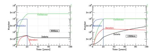
Figure 22: The solution of Equation 5-22 for  $\lambda = 2000/\text{yr}$  at 600 km (left panel) shows the decay from atmospheric drag if the live satellites are all removed after 20 years. By contrast the right panel shows the solution for 1200 km, where the debris density continues to rise for the atmospheric drag time of 500 years.
