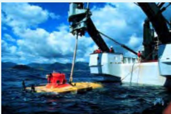
**The R/V Kaimikai-O-Kanaloa is the mothership for the Pisces V submersible. The vessel has accommodations for 10 scientists and a range of 15,000 nautical miles or 50 days. This ship will allow MarBEC researchers to access remote ocean locations throughout the Pacific.**
