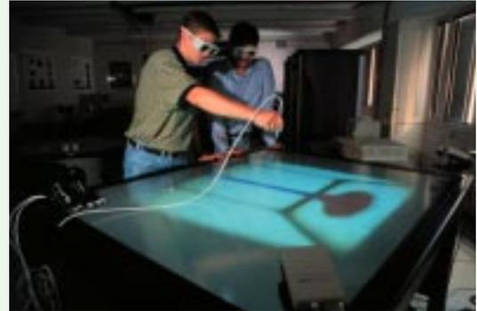
**Center research teams simulate the molecular structure of fibers and films in a virtual environment with the Concurrent Technologies Virtual Workbench. Contact gloves, joysticks, and electromagnetic tracking devices are used to navigate through the three-dimensional scene.**
