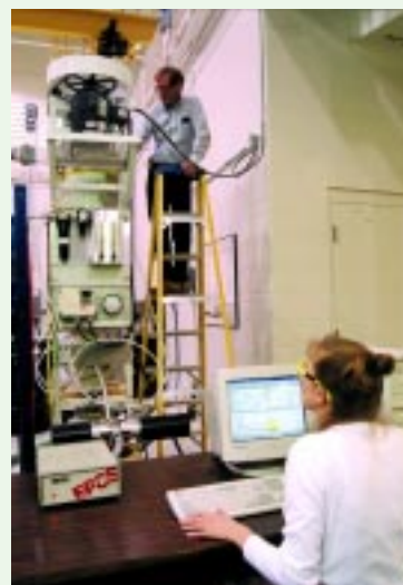
ERC Graduate student and CRIT Engineer conducting research on an ERC-developed particle classifier using an on-line particle sizer.
