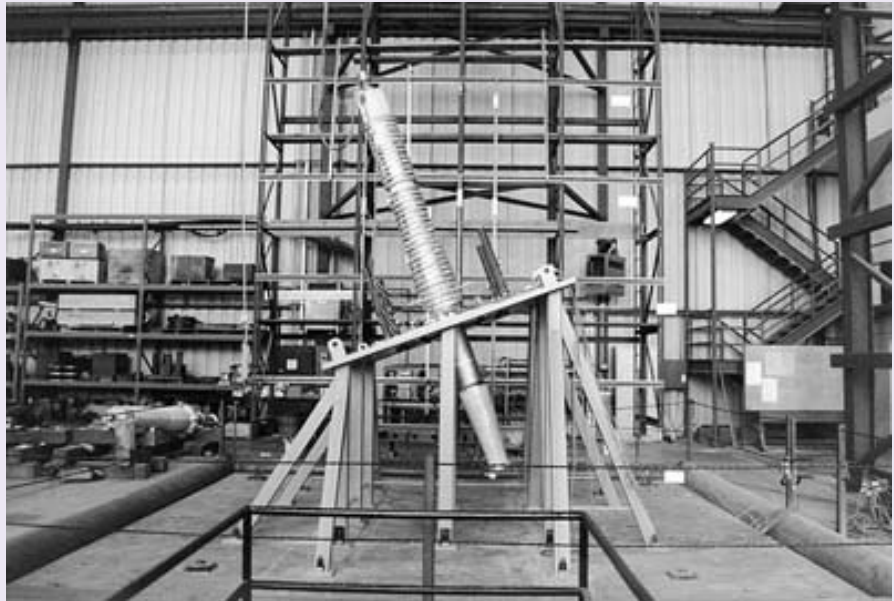
Earthquake simulator testing of utility lifeline equipment
