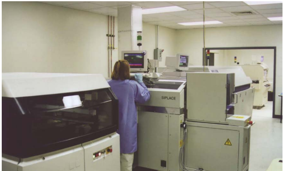
Automated electronics assembly line.
