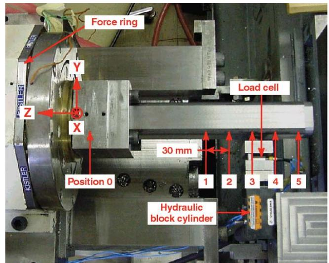
Sensor Integration in a Spindle Housing of Milling Machine.
