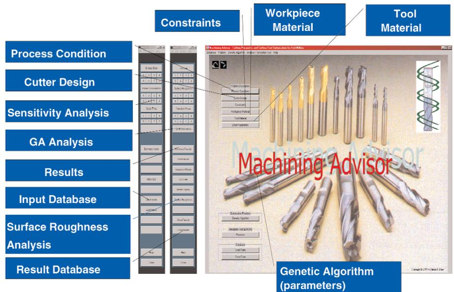
The initial screen of the Machining Advisor software (featured in June 1999 issue of *Cutting Tool Engineering*) that can generate process parameters that simultaneously satisfy economic, productivity, and quality design constraints, while providing sensitivity analysis allowing the user to make necessary trade-offs.
