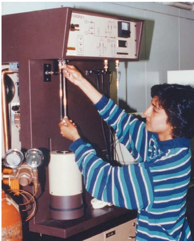
**The Center emphasizes principles of materials science and application to pharmaceutical processing. Here, a graduate student measures the surface area of a pharmaceutical powder.**
