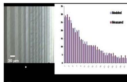
Professors Eric Baer and Anne Hiltner, a method has been devised to fabricate such films that have a continuously varying layer thickness. This technology produces polymer films with previously unattainable, large differences in layer thickness distributions. Gradient films with layer thickness distributions in the nanometer scale possess wide optical reflection bands that may be used as light enhancers, filters, and reflectors in electronic and informational devices.
