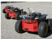
Page 50: These robots are part of the multi-robot testbed and include a custom suite of sensing, computing and communication equipment. Experiments using these robots range from demonstrating control systems that move the robots in formation to a spoken dialogue interface that allows a single operator to command the robots through normal speech.
