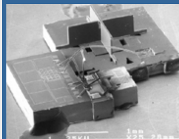
This "Golem Dust" mote is a sensor that detects ambient light and acceleration, and incorporates a tiny radio antenna (the cross) for communication.
