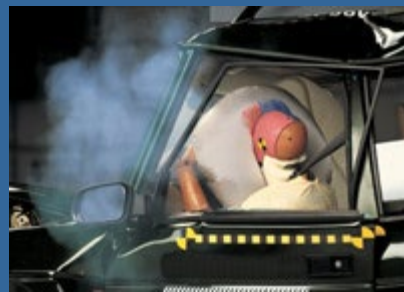
Air bag deployment is controlled by precise but inexpensive accelerometers—sensors that detect sudden impacts. The devices are among the most widely used Micro-Electro-Mechanical Systems (MEMS).
