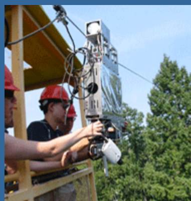
A robotic sensor package is suspended between two treetops at the Wind River Canopy Crane Research Facility in Washington State. The instrument can move along the cable as well as up and down, providing images and precise local climate data.
